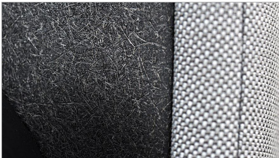
Exhibit 17: Natural fibres used in BMW i3 interior
